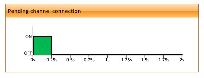
If the edge resistance is above normal, due to lack of/improper termination or cable damage, the offending channel's LED will turn on for 0.25 seconds, 2x per cycle.
