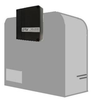
NOTE: It is recommended to place the RX in a location where there is clear, line of site, between the RX and all of its TXs. This can be accomplished by extending the top of the RX approximately 1" above the top edge of the operator, mounting on top of the operator, or on a side that is in line of site with both edge transmitters.
