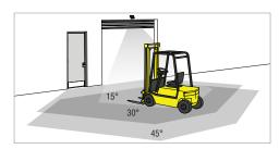
Scenario 1: Vehicle approaches: Vehicle-detection relay is activated. Door opens. Person-detection relay is not activated. Entrance for people remains locked.
