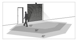
Scenario 2: Person approaches: Vehicle-detection relay is not activated. Door remains closed. Person-detection relay is activated. Entrance for people unlocks.
