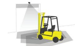
Vehicle approaches: Vehicle-detection relay is activated. Door opens.
