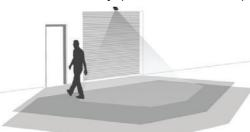
**Person approaches:** Vehicle-detection relay is not activated. Door remains closed. Person-detection relay is activated. Entrance for people unlocks.
