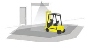
Vehicle approaches: Vehicle-detection relay is activated. Door opens. Person-detection relay is not activated. Entrance for people remains locked.
