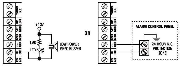
The Duress Output will switch to (-) ground when duress code is entered. You may use it to turn ON an LED lamp and /or a small buzzer to notify a guard; or connect it to a 24 hour Normally Open protection zone of an alarm system.
