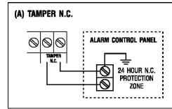
The tamper switch is Normally Closed while the keypad is secured on gang box. It is open when the keypad is removed from the gang box. To prevent sabotage, connect these terminals in series with a 24 hour N.C. protection zone of an alarm system if required.
