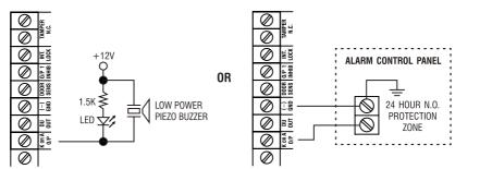
The Alarm Output switches to (-) ground in door forced to open or the door open after Egress Delay. You may use it to turn ON an LED lamp and/ or a small buzzer to notify a guard; or connect it to a 24 hour Normally Open protection zone of an alarm system. See Location 80 and Location 91 for more information about these functions.
