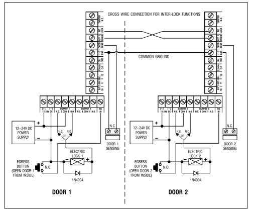
An inter-lock system needs two door controllers. This application example uses two keypads with simple cross wire connection on their "Output 1 Inhibit" and "Inter-lock Control Output" terminals. It is necessary to link up the "(-) GND" terminals of the two keypads as common ground to achieve the inter-lock logical functions.
