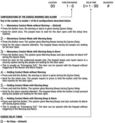
Output 1 activates instantly (the door is released instantly) when the Egress Button is pressed.
