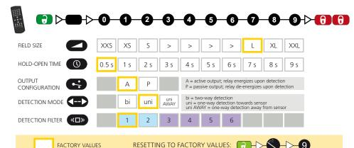
The vehicle detection filter increases the response time of the sensor.
