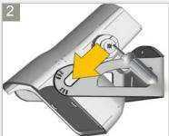
Position the sensor on the bracket and fasten the screws firmly.
